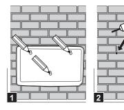
3 Mount the rear casing to the wall with the screws and plugs from the accessory bag.
