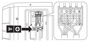
5 Tighten the terminal screws securely. We recommend using a Phillips screwdriver.
