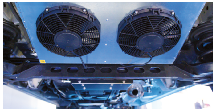
Installation of the SFZ 009e condenser in the back of the vehicle.
