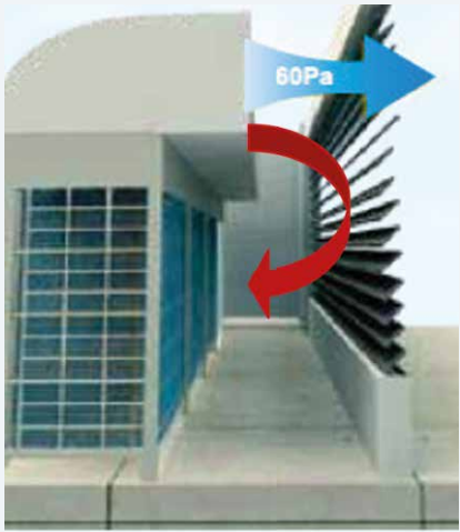
Example of an enclosed installation with downward louvers, preventing proper system functioning
